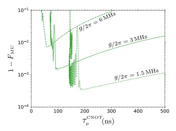
FIG. 20. CNOT gate infidelity  $1 - F_{MU}$  versus duration  $\tau_{\rm p}^{\rm CNOT}$  for  $\Delta/2\pi = 190$  MHz and several values of the qubit-qubit coupling:  $g/2\pi = 1.5, 3$ , and 6 MHz. The other parameters are the same as in Fig. 18.
