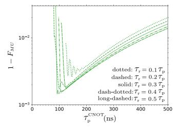
FIG. 21. CNOT gate infidelity  $1-F_{MU}$  versus duration  $\tau_{\rm p}^{\rm CNOT}$  for  $\Delta/2\pi=190$  MHz and several values of the relative duration of the pulse ramps:  $\tau_{\rm r}/\tau_{\rm p}=0.1$  (dotted line), 0.2 (dashed line), 0.3 (solid line), 0.4 (dash-dotted line), and 0.5 (long-dashed line). The other parameters are the same as in Fig. 18. The lines are cut at the left for clarity.
