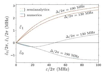
FIG. 6. Effective drive amplitudes  $\tilde{\epsilon}_0$  and  $\tilde{\epsilon}_1$  as functions of  $\epsilon$ , calculated numerically (solid lines with symbols) and using the semianalytical approach (26)–(29) (dashed lines, practically coinciding with the solid lines). We used  $g/2\pi=3$  MHz,  $\eta_c/2\pi=\eta_t/2\pi=300$  MHz, and two values for the detuning:  $\Delta/2\pi=130$  and 190 MHz.
