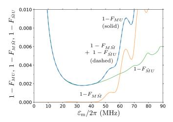
FIG. 15. Decomposition of the CNOT gate infidelity  $1-F_{MU}$  (solid blue line) into the leakage contribution  $1-F_{M\bar{M}}$  (orange line) and contribution  $1-F_{\bar{M}\bar{U}}$  due to imperfect unitaries (green line). The sum  $(1-F_{M\bar{M}})+(1-F_{\bar{M}\bar{U}})$  (dashed blue line) is practically indistinguishable from the solid blue line. We use  $\Delta/2\pi=130$  MHz and the parameters from Fig. 14.
