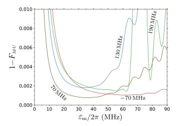
FIG. 14. Infidelity  $1-F_{MU}$  of the CNOT-equivalent gate as a function of midpulse drive amplitude  $\varepsilon_{\rm m}$  for several values of detuning:  $\Delta/2\pi=-70$  MHz (red line), 70 MHz (brown line), 130 MHz (blue line), and 190 MHz (green line). The other parameters are  $g/2\pi=3$  MHz,  $\eta_{\rm c}/2\pi=\eta_{\rm t}/2\pi=300$  MHz,  $\omega_{\rm d}=\omega_{\rm t}^{\rm c0}$ , and  $\tau_{\rm r}/\tau_{\rm p}=0.3$ .
