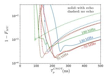
FIG. 23. CNOT gate infidelity  $1 - F_{MU}$  versus duration  $\tau_p^{\text{CNOT}}$  for the echo-CR gate (solid lines) and the basic CR gate (dashed lines). The detunings  $\Delta/2\pi$  are 190 MHz (green lines), 130 MHz (blue lines), 70 MHz (brown lines), and -70 MHz (magenta lines). The parameters are the same as in Fig. 18, except we use  $\omega_d = (\omega_t^{c0} + \omega_t^{c1})/2$ . The lines are cut at the left for clarity.
