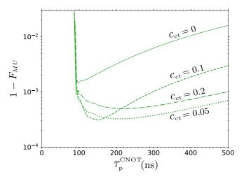
FIG. 22. CNOT gate infidelity  $1 - F_{MU}$  versus duration  $\tau_{\rm p}^{\rm CNOT}$  for  $\Delta/2\pi = 190$  MHz and several values of the microwave crosstalk coefficient:  $c_{\rm ct} = 0$  (solid line), 0.05 (dotted line), 0.1 (dashed line), and 0.2 (dash-dotted line). The other parameters are the same as in Fig. 18. The lines are cut at the left for clarity.
