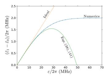
FIG. 5. The CR gate speed  $\tilde{\epsilon}_1 - \tilde{\epsilon}_0$  as a function of the drive amplitude  $\epsilon$ , calculated using the linear-order approximation (19) (dashed straight line), third-order approximation (38) and (41) (solid green line), and numerically (solid blue line with symbols). The parameters are the same as in Fig. 4.
