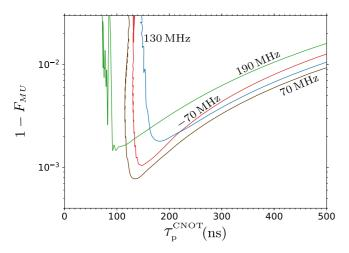
FIG. 18. Parametric plot for the CNOT gate infidelity  $1-F_{MU}$  versus the CNOT gate duration  $\tau_{\rm p}^{\rm cNOT}$  (the running parameter is  $\varepsilon_{\rm m}$ ) for the detunings  $\Delta/2\pi=-70$ , 70, 130, and 190 MHz. We assume  $g/2\pi=3$  MHz,  $\eta_{\rm c}/2\pi=\eta_{\rm t}/2\pi=300$  MHz,  $\omega_{\rm d}=\omega_{\rm t}^{\rm c0}$ , and  $\tau_{\rm r}/\tau_{\rm p}=0.3$ .
